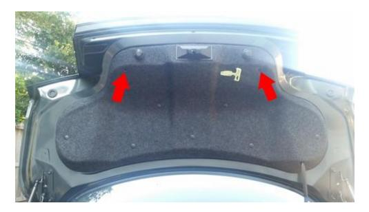
Step 3. Remove stock plastic rivet.
